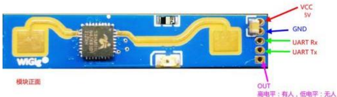
Figure 1 Module pin definition diagram
